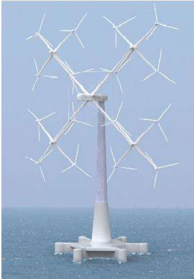
Greenward CTO Ed Salter says the 16-unit array could generate up to 20 MW
