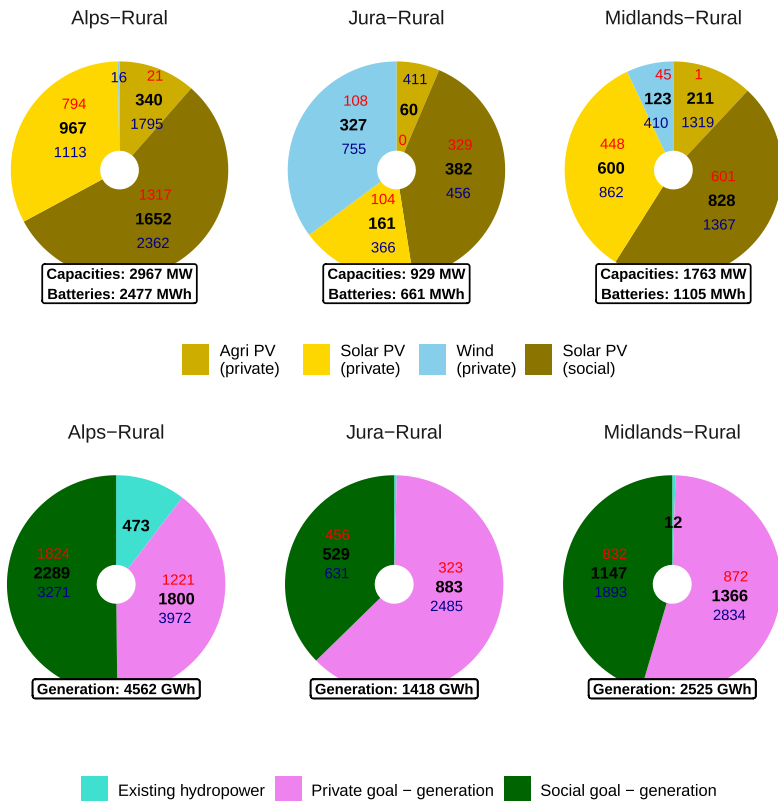
Figure 3 : Optimal renewable generation capacities and storage (top) and expected generation outputs (bottom) from rural LECs in 2035 in the Alps, Jura and Midlands for the median demand scenario. The distinction is made between capacities and generation from optimizing the private objective of return on investment (first stage of the algorithm), and the additional generation capacities and storage added under the social objective (second stage)
